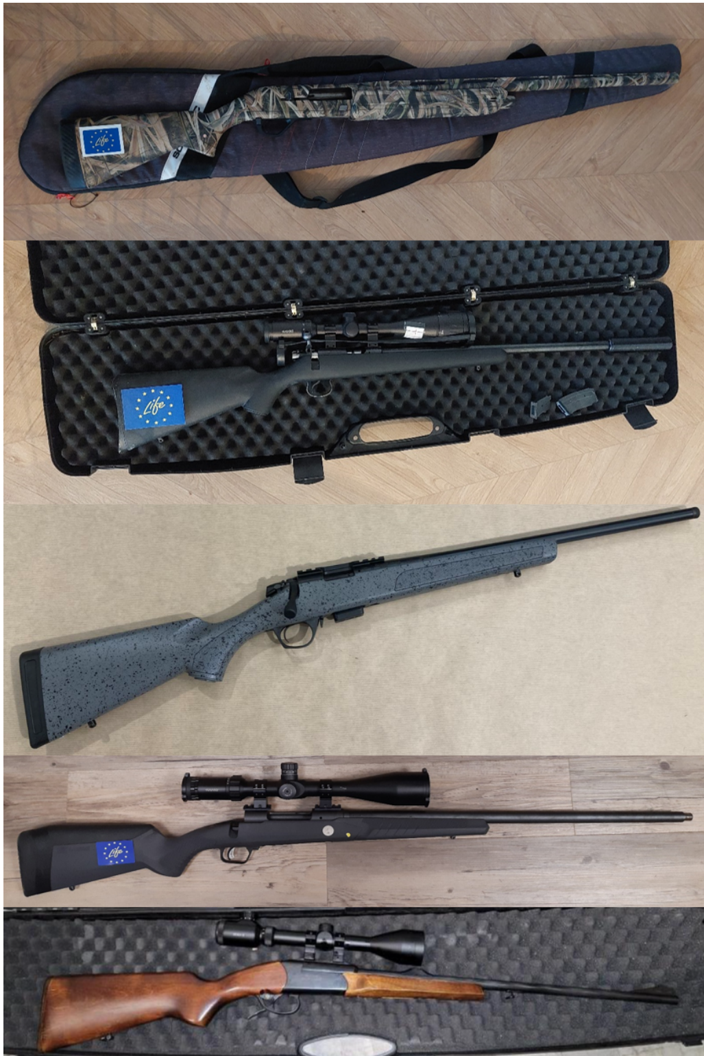
Figure 10: Weapons used. (a) smoothbore rifle caliber 12 cambered 89; (b) .22 long rifle carbine; (c) .17 HMR carbine; (d) .22-250 carbine; (e) .222 carbine
